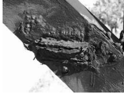
Exfoliation of carbon steel
